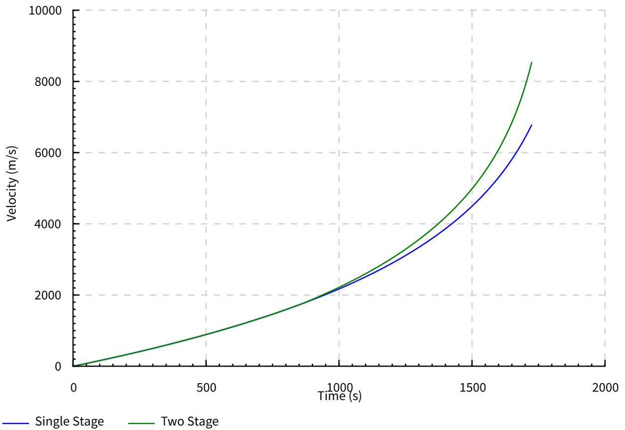
**Figure 3.1:** Velocity profile of the different staging scenarios. The two-stage rocket achieves a substantially higher final velocity despite the same propellant mass.
