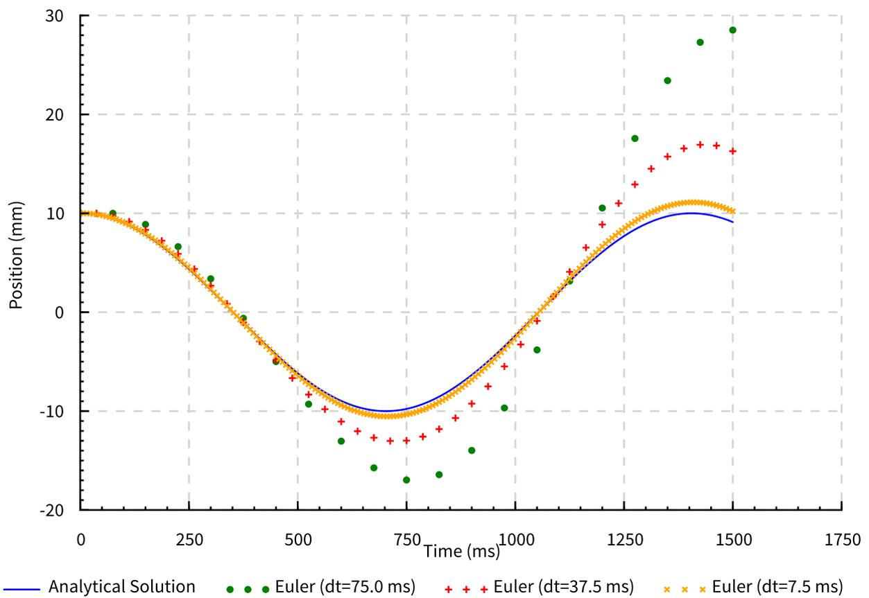
**Figure 2.2:** Comparison of Euler integration with the analytical result for the position variable of a simple harmonic oscillator. The solid line shows the analytical solution while the points demonstrate the Euler approximations for different time steps.
