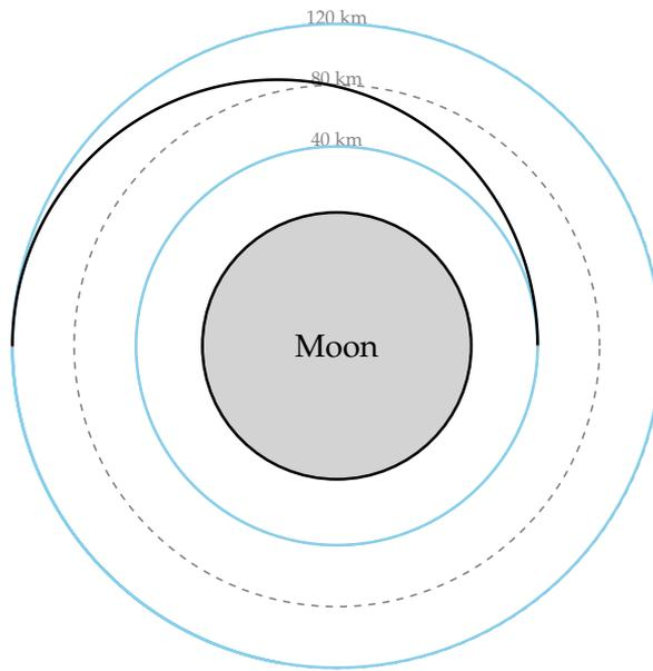
**Figure 4.6:** High impulse Hohmann transfer numerical simulation, using parameters representative of a chemical rocket. The burn trajectories (shown in red) are so short as to be invisible. The altitude scale is magnified by a factor of 20.
