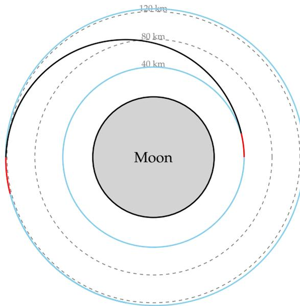
**Figure 4.7:** Low impulse Hohmann transfer simulation. The nominal transfer is from 40 km to 120 km of altitude. The burn trajectories are visible but still short enough that the analytical solution is a good approximation. The altitude scale is magnified by a factor of 20.
