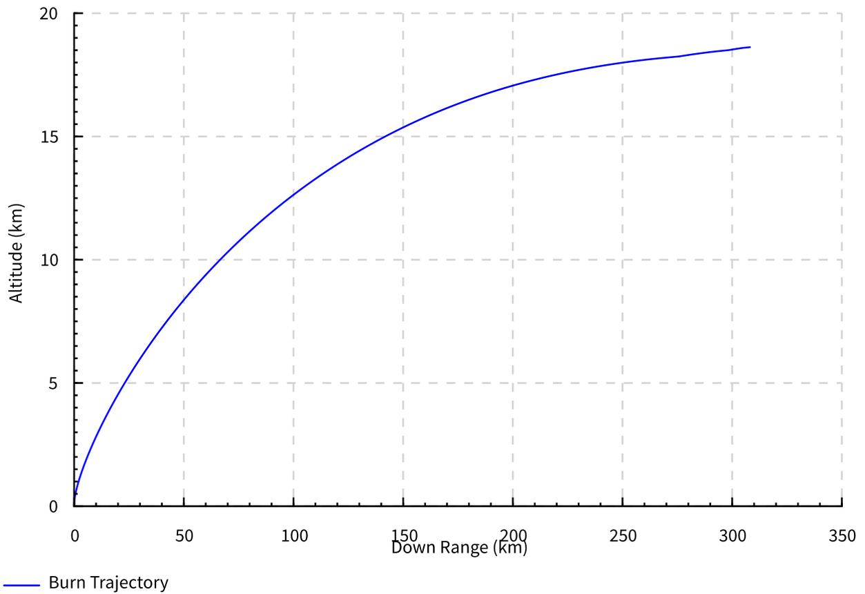
**Figure 2.5:** The entire burn phase of the lunar ascent, shown using altitude-downrange coordinates. The altitude is the radial height above the moon surface, while down-range is the arc-length distance travelled when projected radially downward onto the lunar surface.
