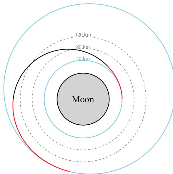
**Figure 4.8:** Ultra-low impulse Hohmann transfer numerical simulation. The nominal transfer is from 40 km to 120 km of altitude. Now the burn trajectories are more substantial and detrimentally affect the final orbit, so that the analytical solution is entirely non-representative of the outcome. The altitude scale is magnified by a factor of 20.
