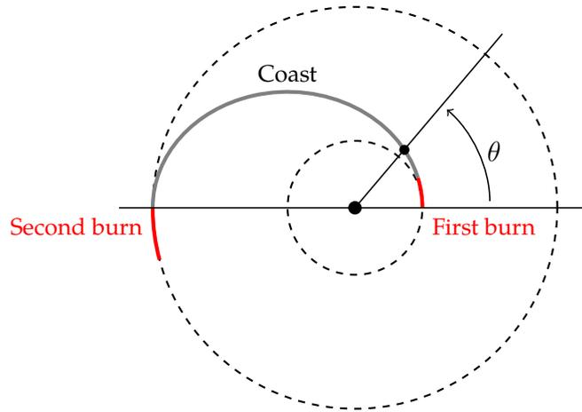
**Figure 4.4:** Simulated burns for the Hohmann transfer (red) and coasting trajectory (black). The first burn will start at  $\theta = 0$ , while the second burn will start at  $\theta = \pi$ . Both burns will be oriented along the instantaneous velocity vector of the craft.
