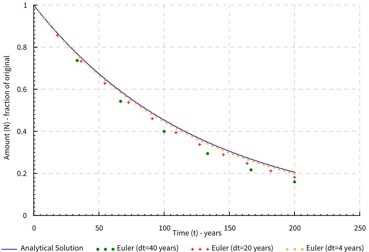
**Figure 2.1:** Comparison of Euler integration with the analytical result for radioactive decay of the isotope  $^{238}\text{Pu}$ . The solid line shows the analytical solution while the points demonstrate the Euler approximation for different time steps.
