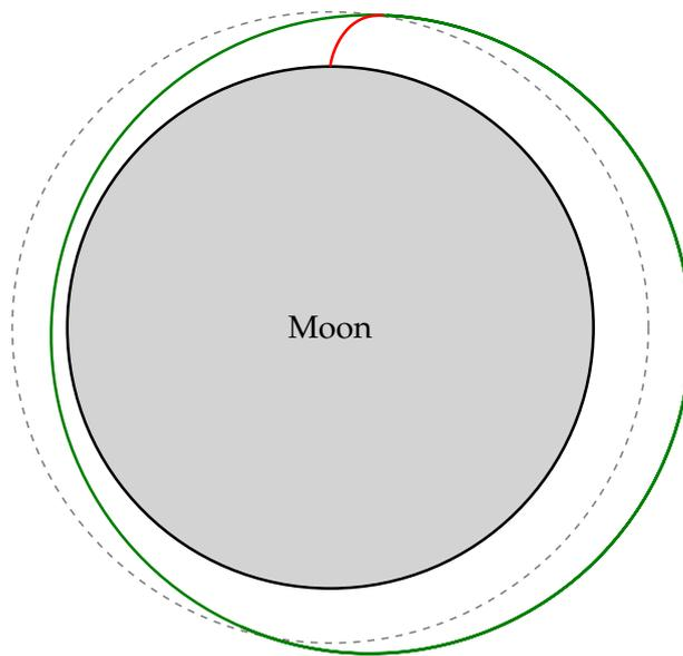
**Figure 2.6:** Moon-centred view of the burn and coasting phases. The radial (altitude) scale above the lunar surface is magnified by a factor of 20. The dashed line shows the target altitude. The target orbit is elliptical, as specified by the target velocity vector, which has a positive radial component.
